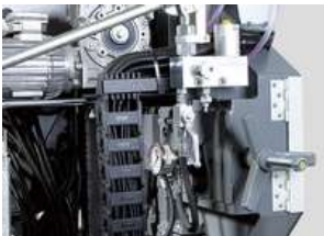
Hydraulic saw blade tensioner
