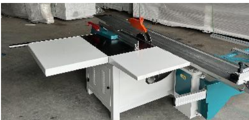
6. The solid outrigger makes it possible to process large and heavy workpieces
