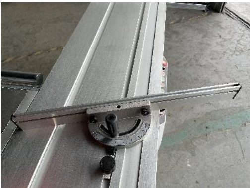
6. The solid outrigger makes it possible to process large and heavy workpieces
