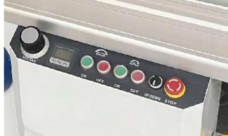
4. Manual tilt handle and control panel(Digital angle readout is optional)
