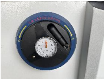
4. Manual tilt handle and control panel(Digital angle readout is optional)
