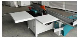
7. The crosscut fence can be attached to the sliding table without the use of tools. The end stop provides you with the exact 90° position.
