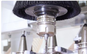
定向吹灰吸尘装置 Directional soot blowing and vacuuming device
