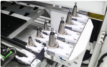
八刀位自动换刀刀库 ATC 8 by servo
