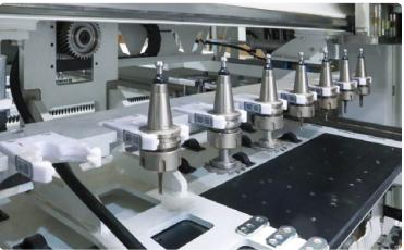
NCB612DPTL配置2组8刀位自动换刀刀库 2 sets 8-slot tool magazine of NCB612DPTL
