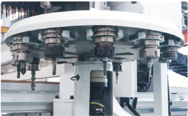
12刀位伺服换刀刀库 ATC 12 by servo
