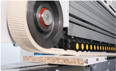
履带压料 Top presser by v-belt
