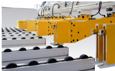
配置10个工夹 10 sets of main grippers
