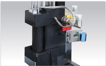
可选: 双色免清洗PUR涂胶 Optional: two-color no-cleaning PUR glue
