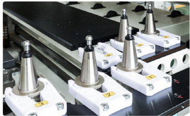
六刀位自动换刀刀库 ATC 6 by servo
