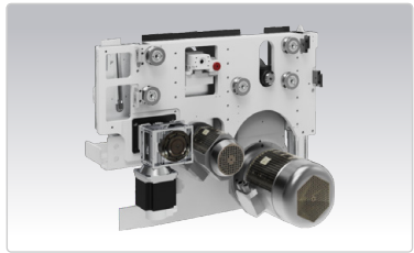
整体式锯座 Integrated saw carriage
