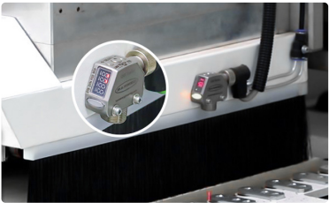
宽度自动检测及补偿 Automatic width detection and compensation
