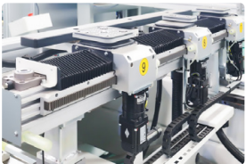
伺服控制梁式台面 Beam Table by servo control
