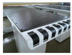
Separate 3 pipes connected to 3 float tables with a 2.2kw air blower beneath the table supplies sufficient air. Flow rate: 5.2m³/min.
