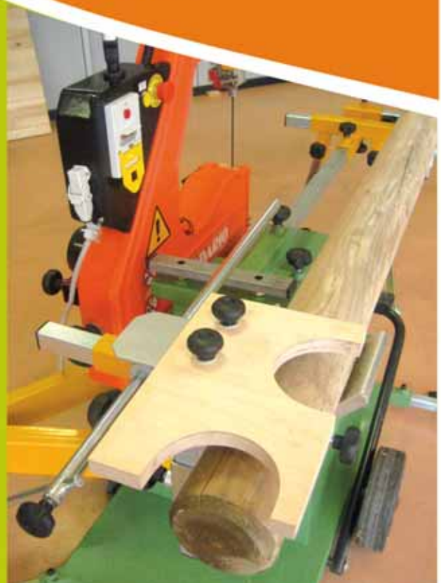
At the side: Set 1500 with application of ST 100 device for cutting trunks
