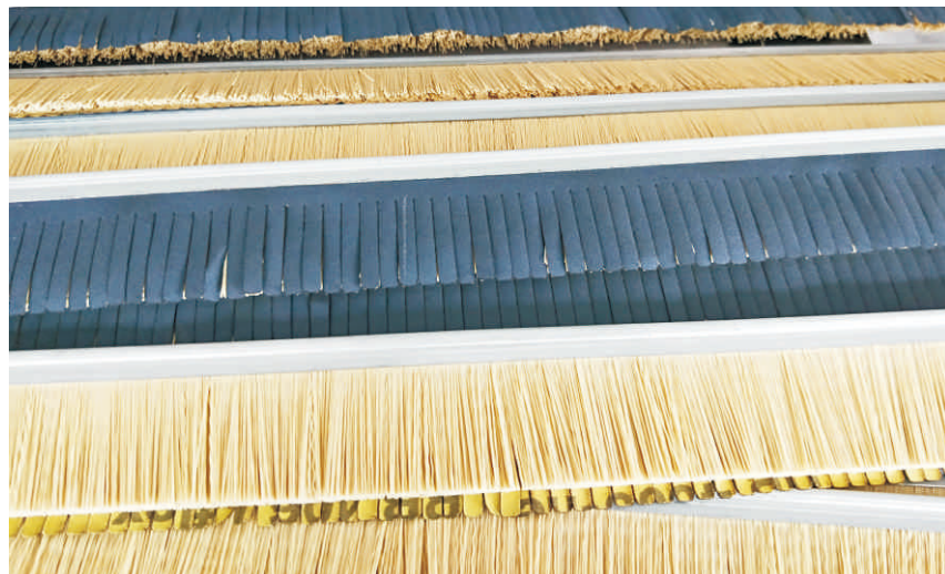
进口砂布剑麻一体式 / Imported sanding paper and brush unit
