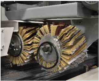
各部件可整体拉出更换磨料快捷方便 Eashly pull out to change consumables
