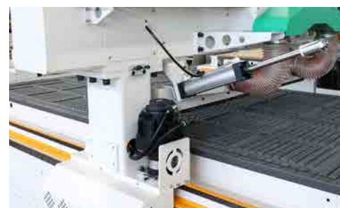
龙门立柱，齿轮齿条闭紧装置 Dragon Gate column, gear rack closed device
