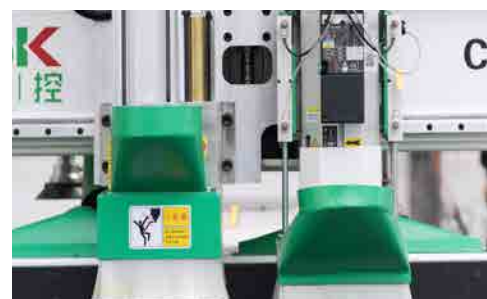
9KW 自动换刀主轴 + (5+4) 9 垂直钻包 9KW automatic sword change spindle+(5+4) 9 vertical drill bag
