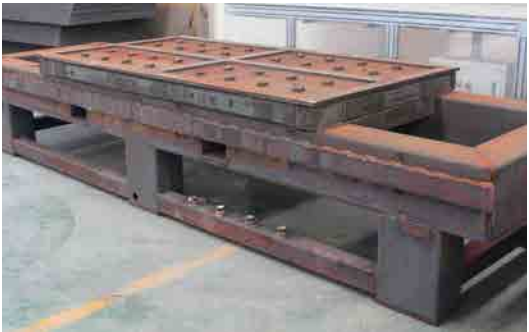
重型床身，钢板台面，时效处理，设备精度高稳定性高 Heavy bed body, steel plate countertop, timeliness processing, high stability of equipment accuracy
