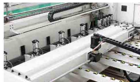
8 套夹手和可升降式压梁 8 sets of hands and lifting beams
