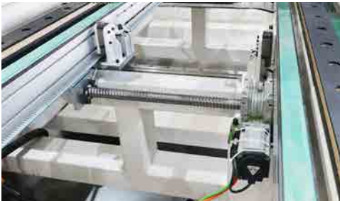
工位宽度自动调节装置 Automatic adjustment device for station width
