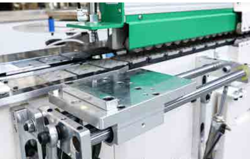
05 窄板辅助送料 Narrow plate assisted delivery
