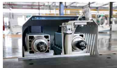
双主轴解决多种生产工艺 Dual spindle to solve a variety of production processes
