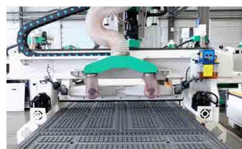
真空吸附台面，推料除尘结构 Vacuum adsorption of the countertop, pushing the dust removal structure
