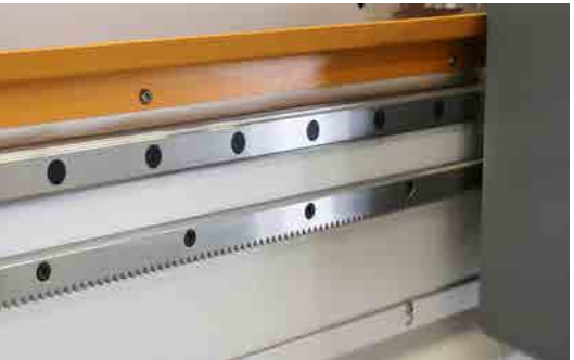
H30 导轨，2M 高精度斜齿，保证设备高速稳定运行 H30 guide rail, 2M high-precision oblique teeth, ensure that the equipment runs high and stable
