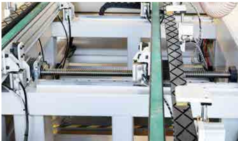
可自动调节工位宽度 Can automatically adjust the width of the station
