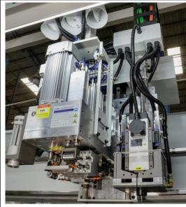
4. Bottom drilling unit and 3.5kw spindle with dust blower device to keep clean.
