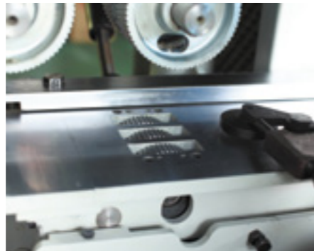
The front work table is equipped with the active feeding wheel material feeding cutoff force.
