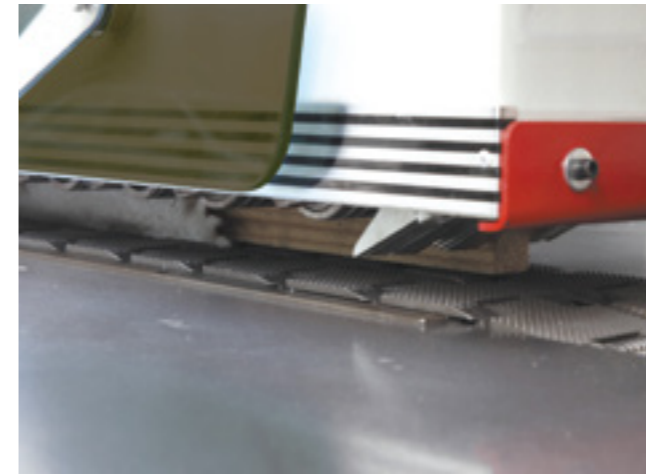
The parts of feeding chain are made by special material and the structure of the teeth is more stronger which will extend the service life and more smoothly in feeding.
