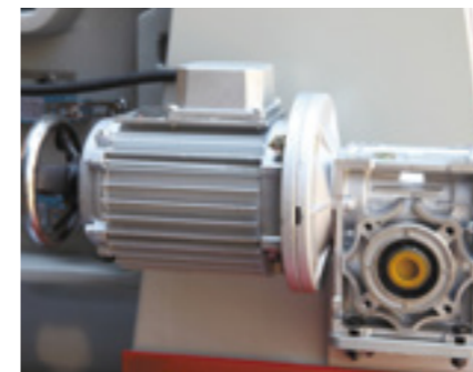
Conveniently adjusting the height with motor.
