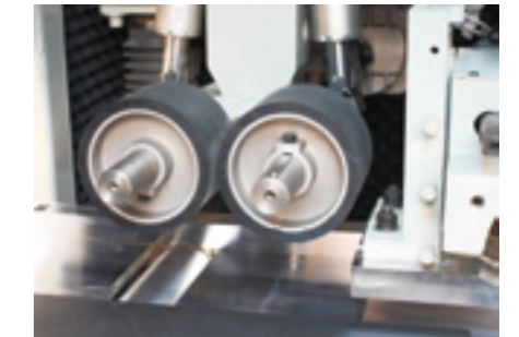
The rear work table is equipped with the active feeding wheel ensuring the smooth feeding.
