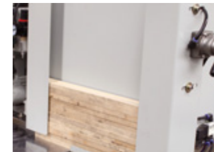
The short material feeding device is optional for the purpose of coovenienting high speed feeding for short workpiece.
