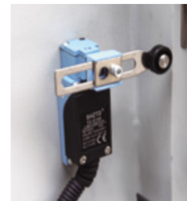
Automatic thickness measurement and lower limit switch.
