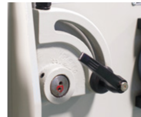
The feeding unit can be adjusted up-wards and downwards,the elevating range reaches 6mm, and thus the processing precision can be enhanced with powerful feeding.
