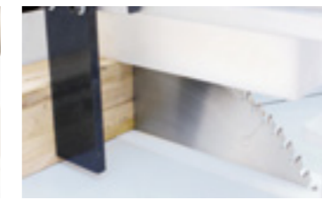
Bottom sawing with high precision
