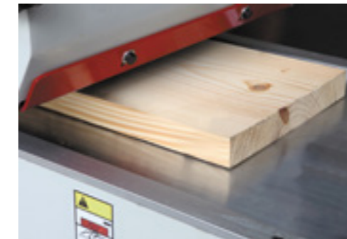
Suitable for double side and fixed-thickness planing for the boards of thickness under 200mm
