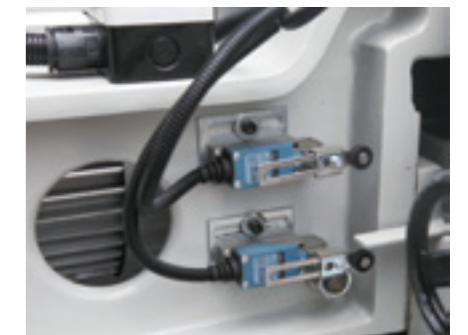
Limited switches ensure the operator safe while saw lifting.
