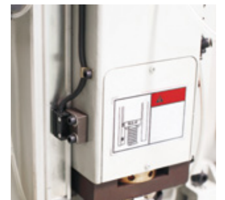
The precision can up to 0.01mm of the magnetic grating digital readout .input the data to set the working thickness automatically.
