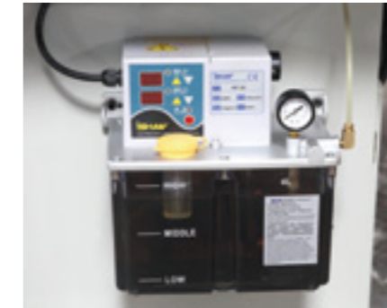
Microcomputer control pump for lubrication of key parts to extend the service life.
