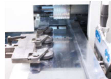
The side infeed device which could ensure infeed smoothly.
