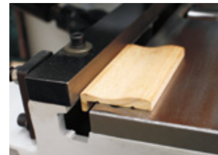
The groove working table is optional for irregular workpiece.
