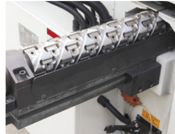
The structure of the bottom cutter shaft can be pulled out quickly .
