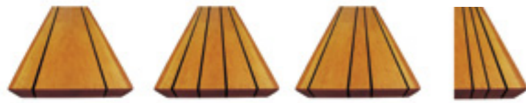
Optimal edge cutting Optimal width cutting Optimal value cutting Apply the second time optimal cutting for the remainder material
