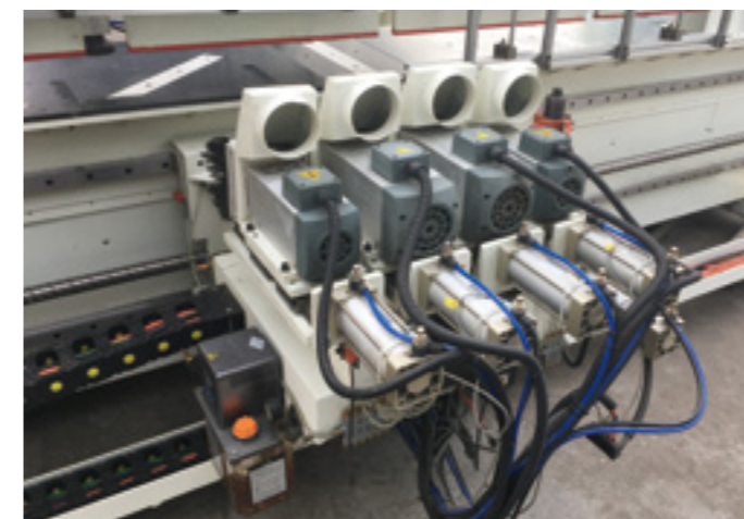
Dust collect for the spindles to keep the working area clean
