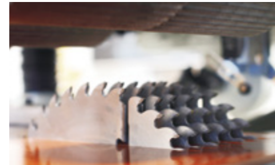
Adopting ultrathin saw blades with low kerf loss which is only 2.6mm and improve wood utilization rate.
