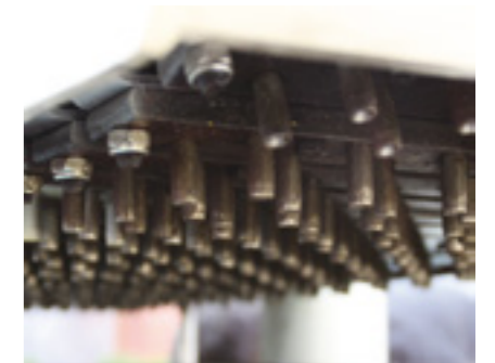
Equipped with pressure plate guarantees short workpiece smooth machining, increasing production output.
