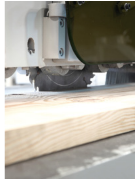
Single-piece longitudinal trimming processing for workpieces with a thickness under 85mm
