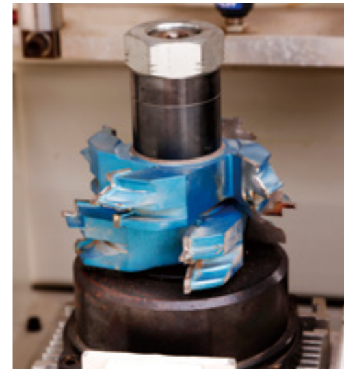
Two high-speed side milling motor spindle, each spindle is equipped with two opposite turning cutters. A high-speed motor spindle for slot milling and drilling
