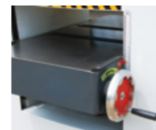
Manul lifting with precision height display
