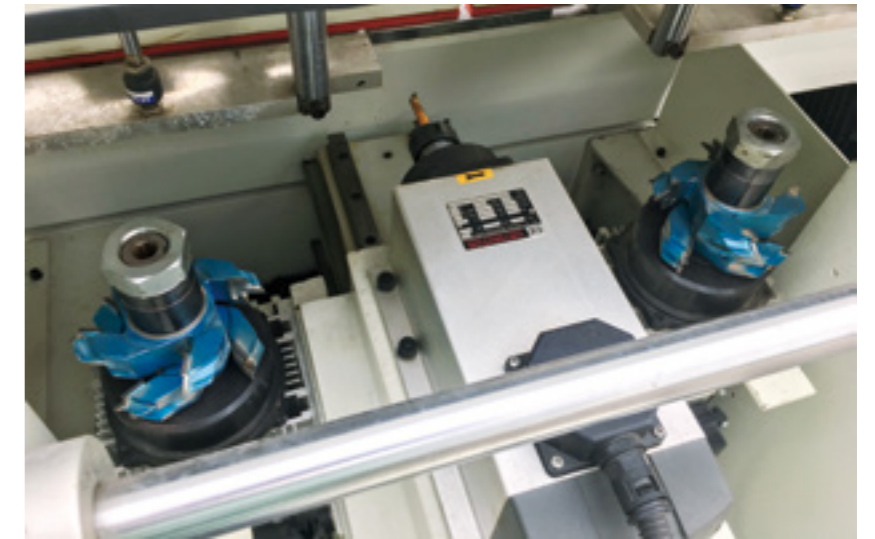
Two high-speed side milling motor spindle, each spindle is equipped with two opposite turning cutters. A high-speed motor spindle for slot milling and drilling
