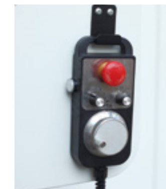
Electronic handwheel for quick and easy tuning
