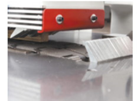
The machine is installed with anti-rebound device on the work table to avoid any material kickback for safety purpose.
