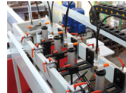
Multi-directional pressure cylinder with fast valve
