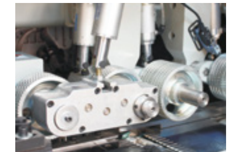
The pressing wheel mechanism for short boards, ensuring the smooth conveying of the short materials (Optional)
