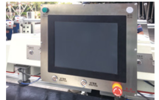
HMI interface, directly input the size in the graphic screen, the operation is simple and easy to learn, and can store 47 data.
