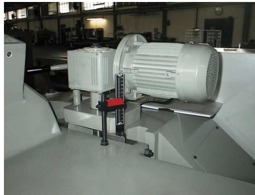
LIFT UP MOTOR WITH INVERTER
